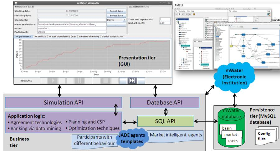
Fig. 1.6 Multi-tier architecture of the *mWater* system
