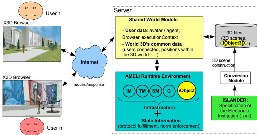
Figure 3. 3D-EI architecture including *iObject* and *iObject3D*
